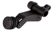
This easy to operate compact window hold-open is designed to fit comfortably using a two finger operation for top and side hinged venting windows for on- and off -highway vehicles. It features an over center design that orientates the window at fully closed and fully open positions and an optional quick release pin in bright red nylon or steel
